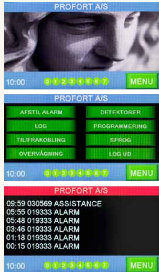
Three screen images from Piccolo Light satellite display: Opening screen, main menu and alarm state.
